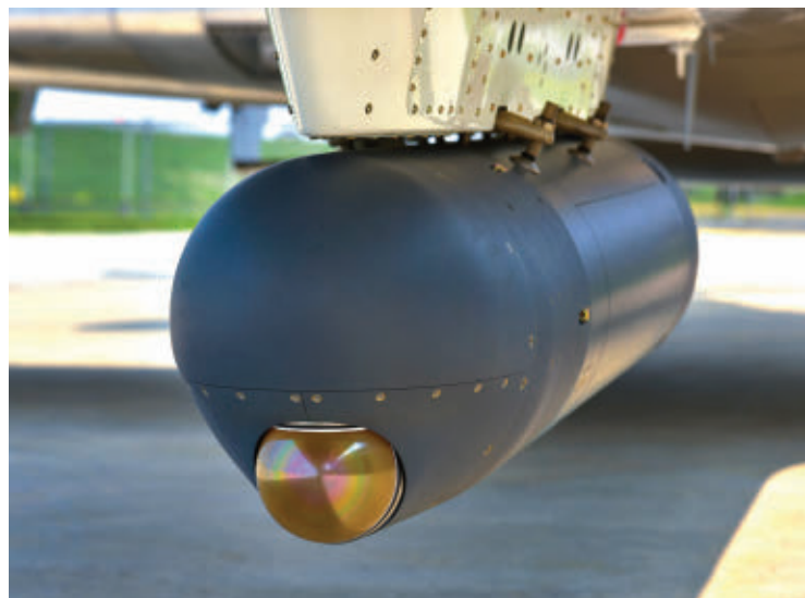
Northrop Grumman is proposing an open-systems architecture for electro-optical sensor pods to ease field maintenance.
