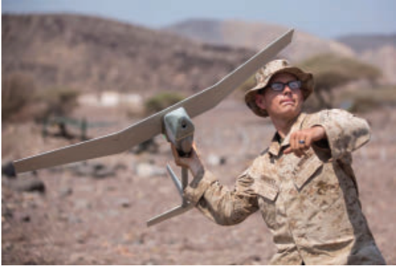
A soldier launches a RQ-11B Raven unmanned aircraft in Djibouti last March. (Marine Corps photo.)
