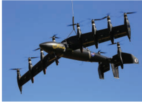
NASA's GL-10 UAS can hover and fly vertically and forward with help from intelligent motor controls. David C. Bowman - NASA Langley
